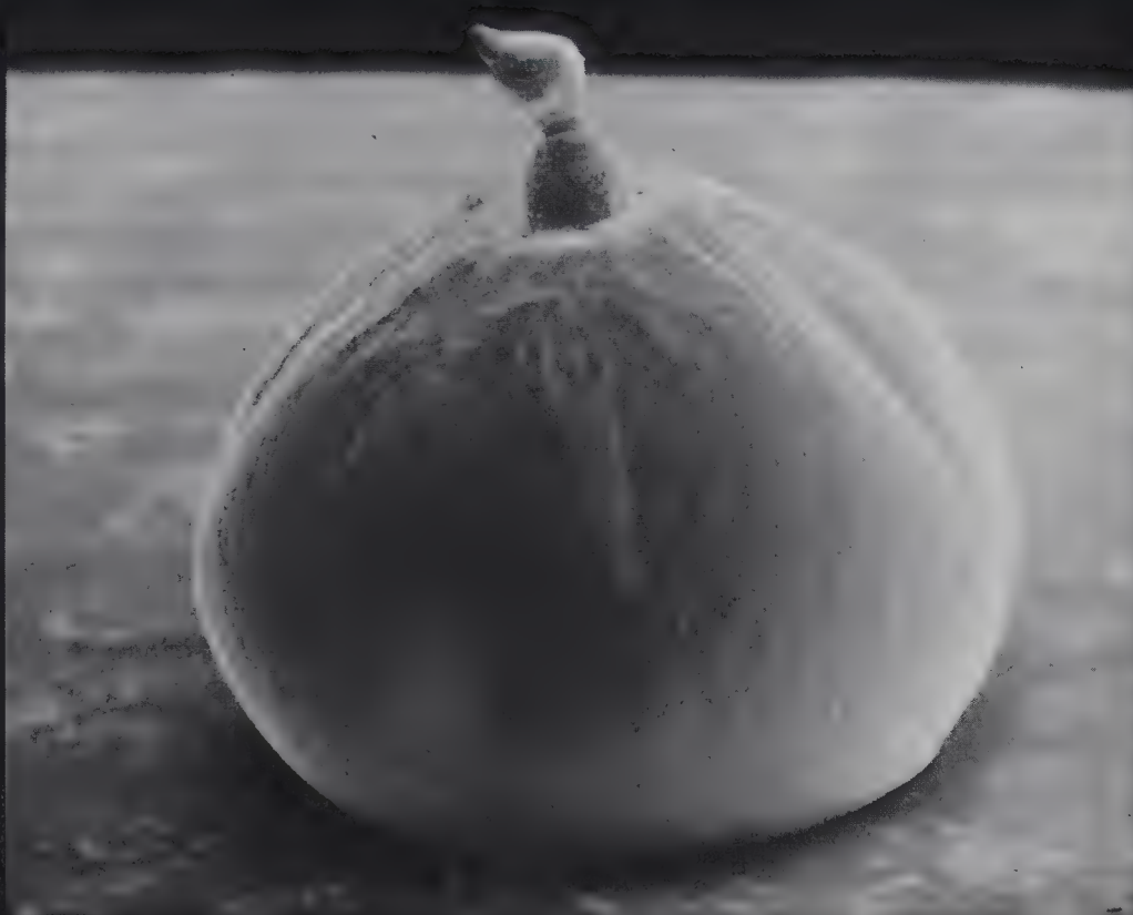
Ball of solder (magnified 35 times)
